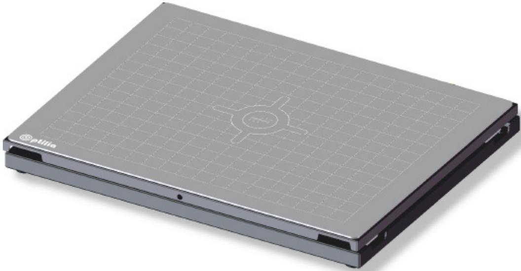
**OP-006 500** is a linear floating XY-translation stage, equipped with thick static dissipative top matting. Ball bearing slider design of the unit permits low friction linear movement with no backlash or side-play. This precision stage provides controlled point-to-point lateral movement along two linear axes. A detachable  $\phi 4$ mm mating plug with 1m flying end wire is included for earth connection.
