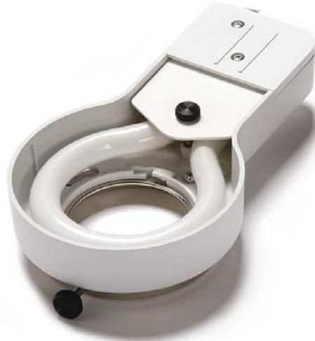
This fluorescence ring-light creates a flicker-free ultra violet illumination. Thanks to its high-frequency control and high quality bulb the ring-light ensures high intensity and very homogenous illumination of the objects. The UV bulb can be easily replaced by a white (daylight) bulb if required.
