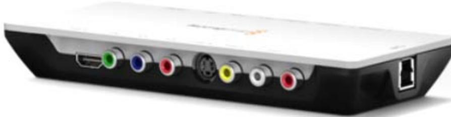
Capture and play back of Full HD uncompressed video via USB3.0. Plug this external Frame Grabber to your PC or Laptop and capture the live image in Full HD digital format in your Optilia OptiPix software. This frame grabber powers from the USB 3.0 connection and is fully DirectShow™ and QuickTime™ compatible.
