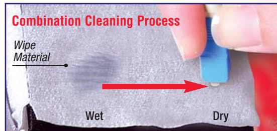
Combination Cleaning™ Process
